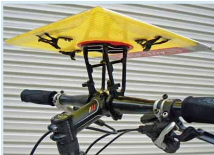
The AutoPilot PilotOne board took my attention with its tool-free fitting that doesn't even include any screws to do up. The two hinged clamps have a long arm that with the use of two adjustable plastic hose clamps tighten on to one of the main uprights. It's hard to explain so I'll include a diagram.
